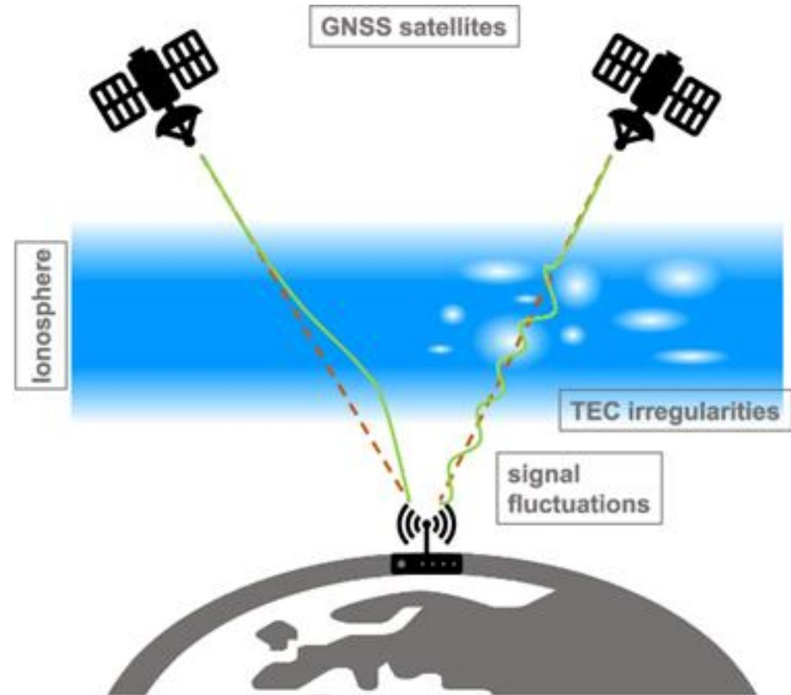
Figure: Scintillation phenomena: the line-of-sight signal path from the GNSS satellites to the receiver on earth (---) and continuous signal accounts for propagation distortions (—) (adapted from Linty et al., 2019)
