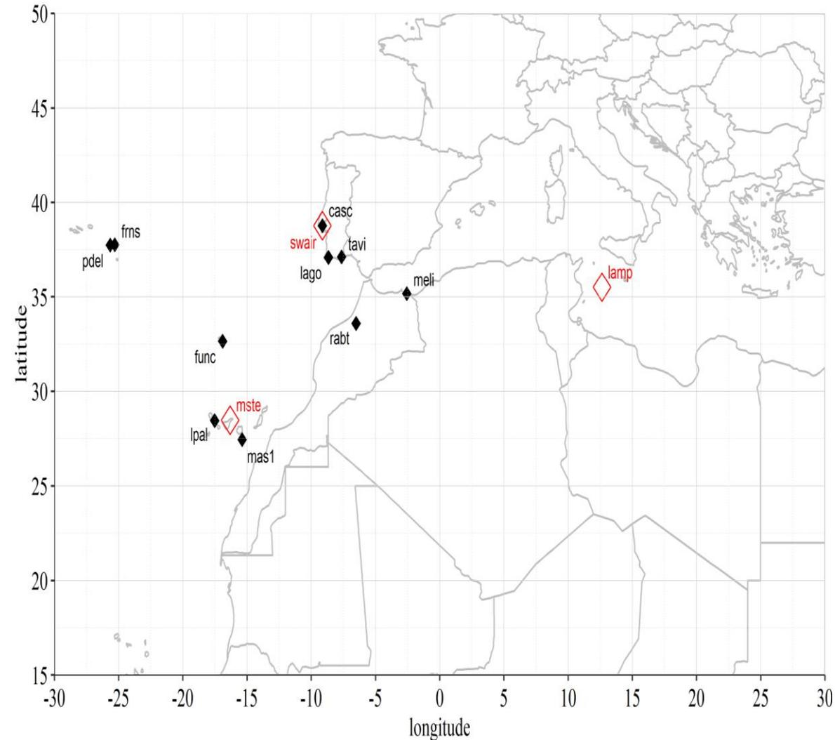
Figure: Locations of GNSS receivers used to calculate S4 (red open diamonds) and ROTI (black diamonds) scintillation indices.
