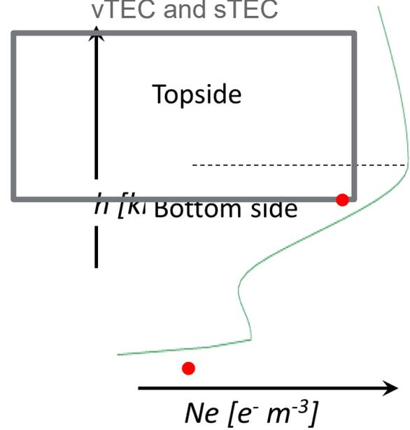
Profiler model - 6 semi-Epstein layers with modeled thickness parameters and is based on anchor points defined by foE, foF1, foF2 and M(3000)F2 values.
