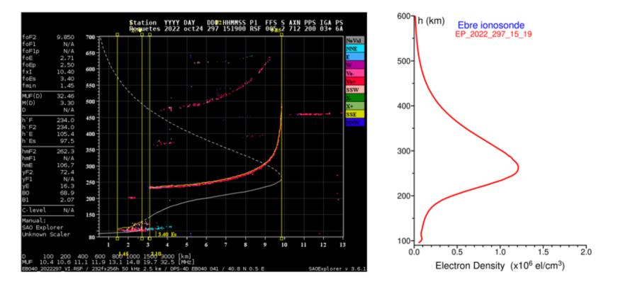
Example (from left to right) of the ground-based HF (ionosonde) sounding recording with results of the ionogram processing, and ionosonde-derived electron density profile Ne(h).
