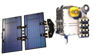
COSMIC-2 RO payload TGRS (Tri-GNSS Radio Occultation Receiver System) developed by JPL RO with GPS and GLONASS signals
