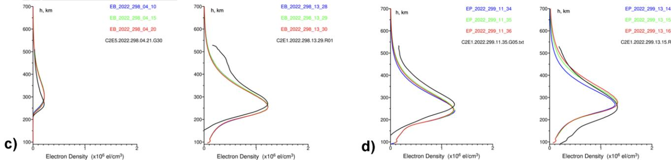
Representative examples of EDP collocation events between COSMIC-2 RO and Ebre ionosonde combining ionogram recording and EDP comparisons for the October 2022 high-rate sounding campaign.
