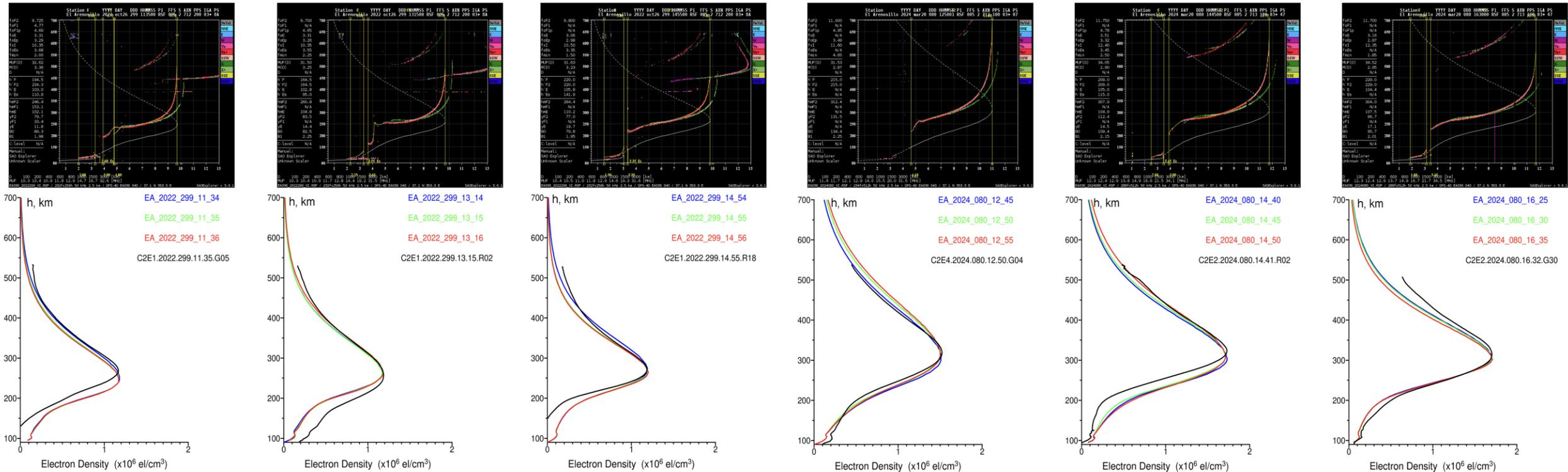
Representative examples of EDP colocation events between COSMIC-2 RO and El Arenosillo ionosonde combining ionogram recording and EDP comparisons for the October 2022 (left) and the March 2024 (right) high-rate sounding campaign.
