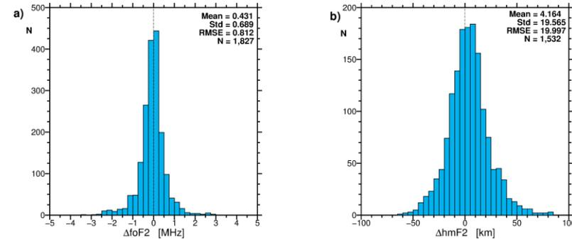
Histograms of the F2 peak parameters residuals  $\Delta foF2$  ( $\Delta foF2 = foF2_{RO} - foF2_{ionosonde}$ ) and  $\Delta hmF2$  ( $\Delta hmF2 = hmF2_{RO} - hmF2_{ionosonde}$ ) between collocated COSMIC-2 and ionosonde measurements
