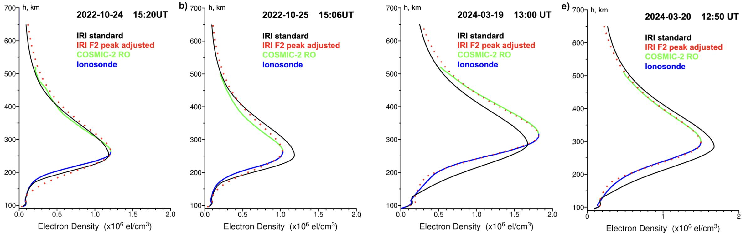
Comparison of the IRI-2020 adjusted EDPs (red dots) with reference combined EDPs (blue-green line). The standard IRI output is shown as a black line.
