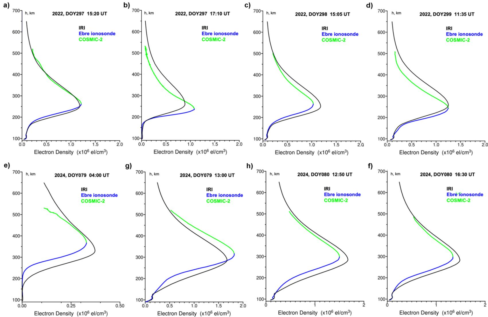
Comparison of the electron density profiles derived from the IRI-2020 (black line) and the reference profiles combined from ionosonde (blue) and COSMIC-2 RO (green) measurement.
