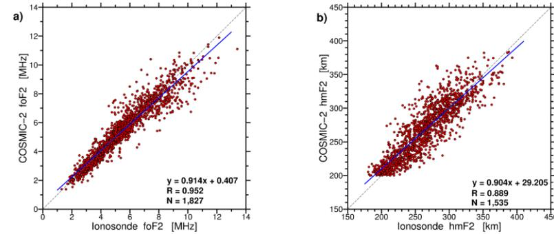
The scatter plots of the COSMIC-2 RO-based foF2 and hmF2 values against the corresponding ionosonde-derived ones.
