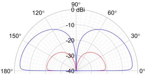
Fig. 10 Antenna gain versus elevation angle of a 2.4 m long vertical whip antenna above average ground ( $\sigma = 5$  mS/m,  $\epsilon_r = 13$ ). The blue curve is for 9 MHz, the red curve is for 3 MHz.
