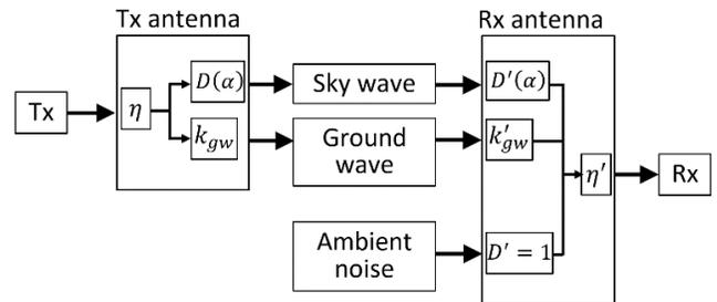
Fig. 6 Block diagram of the radio link (single-ended).
