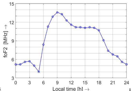
Fig. 3  $f_oF2$  [MHz] vs Local time [h] → red in June in Ilorin, Nigeria, during a solar cycle maximum. Figure adapted from [17].
