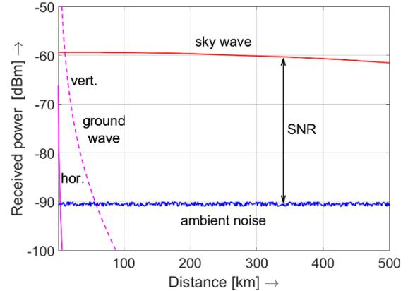
Fig. 2 Ground wave, skywave and radio noise for a 100-Watt transmitter, assuming and lossless isotropic antennas over average ground ( $\sigma = 5$  mS/m,  $\epsilon_r = 13$ ). Frequency is 9 MHz, 14:00 LT, rural area in West-Africa.
