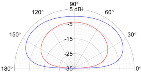
Fig. 8 Antenna gain versus elevation angle of a 37 m (120 ft) long T2FD antenna, 12 m above average ground ( $\sigma = 5$  mS/m,  $\epsilon_r = 13$ ). The blue curve is for 9 MHz, the red curve is for 3 MHz.
