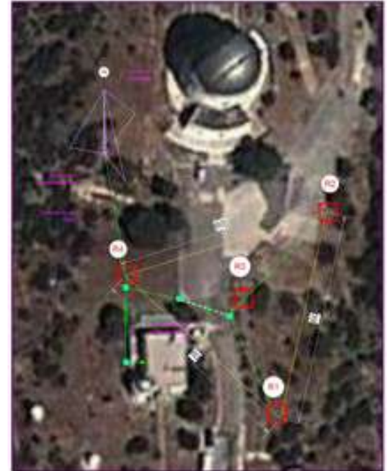
Geometry of the Athens DPS4D installation
